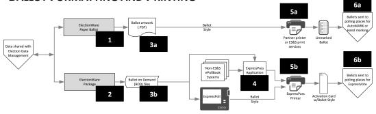
Figure 3: Ballot Formatting and Printing Subsystem
