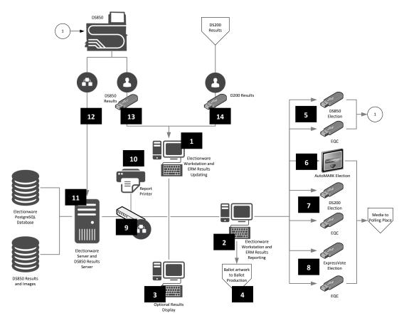
Figure 8: Local EMS Network with Multiple Workstations
