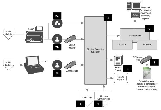
Figure 6: Results Consolidation and Reporting Subsystem
