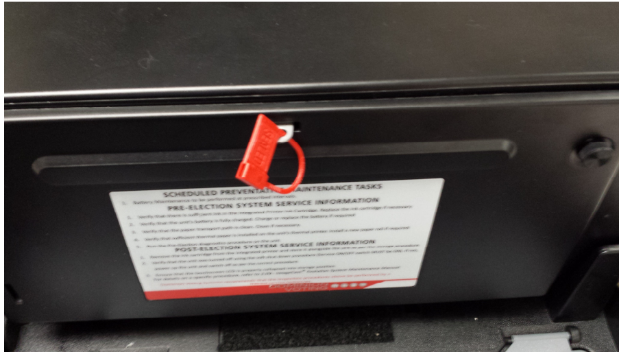
Figure 6 - ICE Scanner Ballot Marking Printer Door Seal in Place
