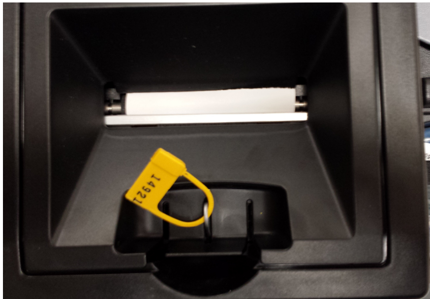
Figure 5 - ICE Scanner Thermal Printer Door Seal in Place
