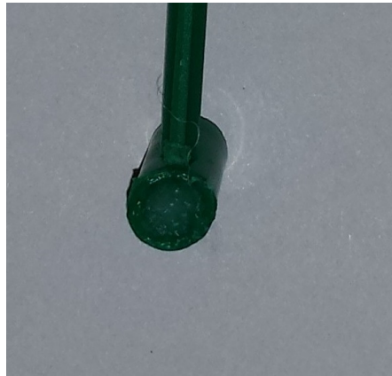
Figure 5 - Plugged End of Hinge-Lock Type Seal
