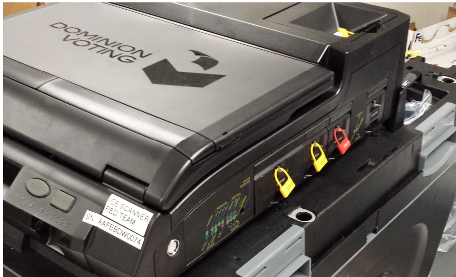
Figure 4 - ICE Scanner Compact Flash Door Seals in Place
