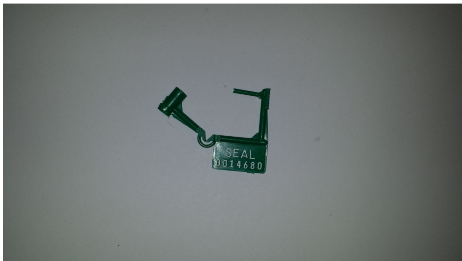
Figure 6 - Broken Hinge-Lock Type Seal
