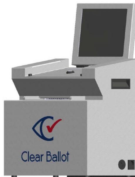
The P1000 will be the first optical scan tabulator built using Intel’s Next Unit of Computing (NUC®)—a high-performance computing platform in a tiny, 4-inch square package. The NUC will enable Clear Ballot to deliver performance (18-inch, 2-sided ballot tabulation in 2.7 seconds) and advanced, out-of-the box functionality with the ability to continue innovation over its 20+ year lifecycle.
