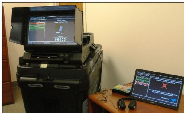
Figure 3. ICE with secondary, “dual” monitor for accessible voting
