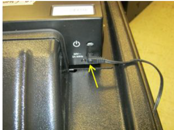
Figure 6-3: Connect the round end of the AC to DC power adapter
