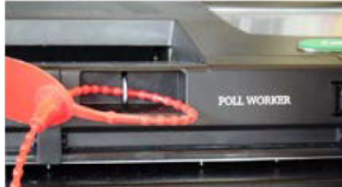
Figure 6-6: Sealing Administrator and Poll Worker Memory Card Access Ports
