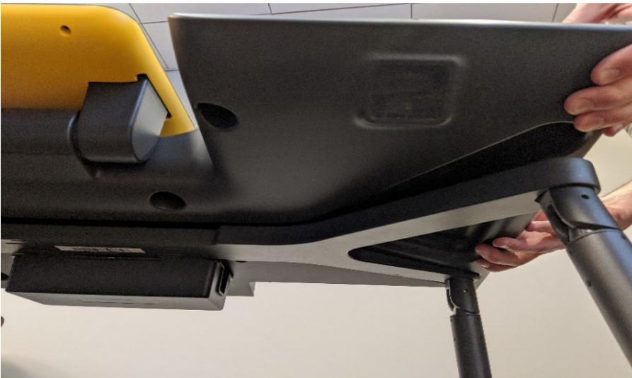
10. Attach the BMD top module to the leg stand by aligning the grooves underneath the BMD top module.
