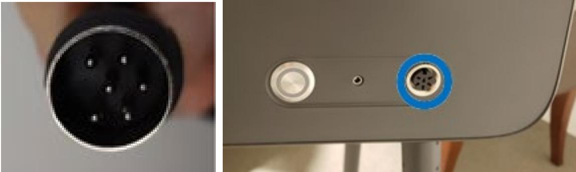
18. Gently insert the six-pronged end of the power cord into the six-pronged socket found on the back of the BMD top module.
