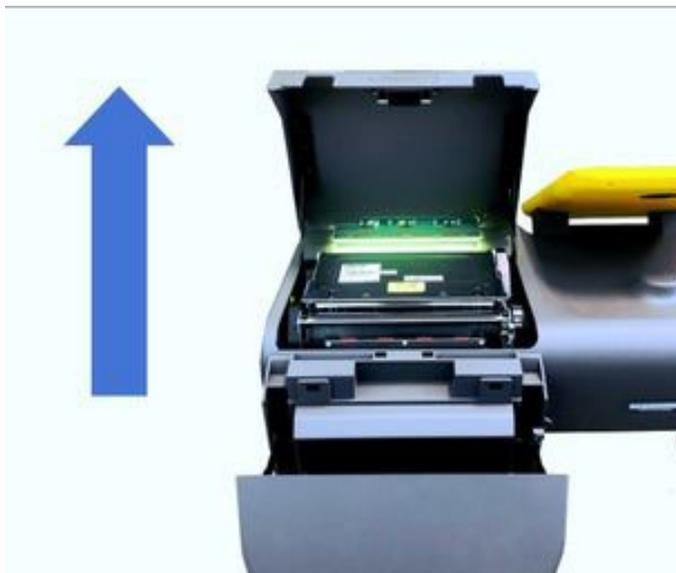
4. Press the button at the center of the plastic printer cover and pull the cover upward.
