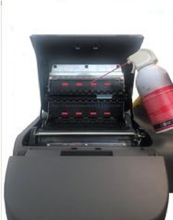
6. Use compressed air to remove external dust.
