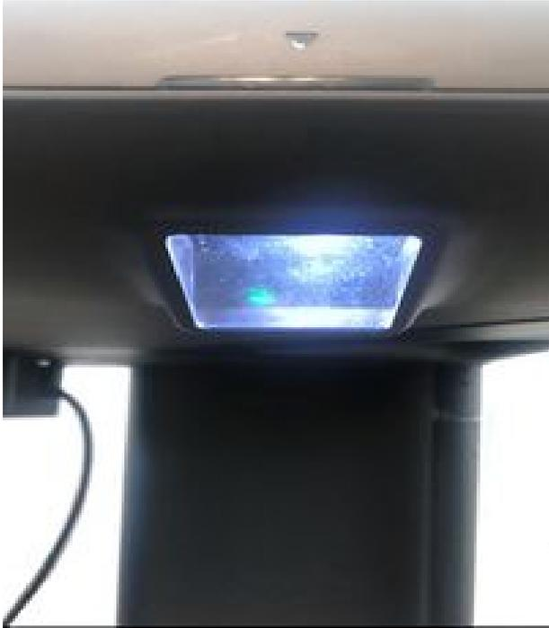
1. To clean the Poll Pass/Security Pass scanner, first locate the glass scanner lens underneath the front right-side of the BMD.
