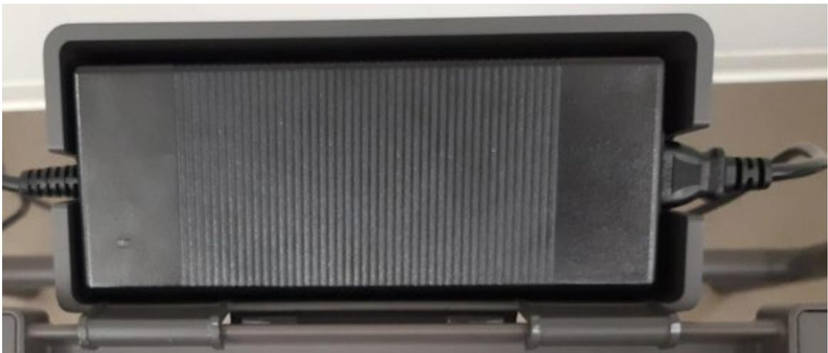
9. Place the power module inside the power bracket, placing the larger power cord in the larger square opening and the smaller cord in the smaller round opening.
