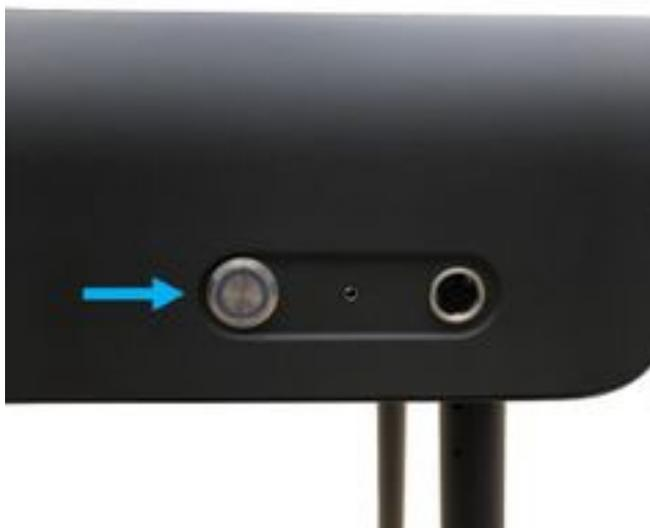
12. Press the Power Button to turn the BMD back on.
