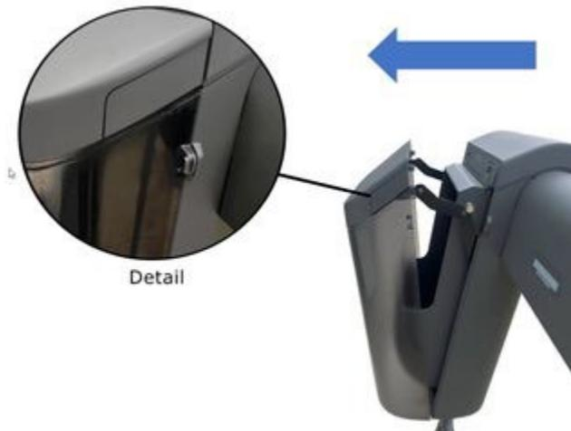
3. Push the button on the upper-left side of the Integrated Ballot Box and pull the back of the Integrated Ballot Box.
